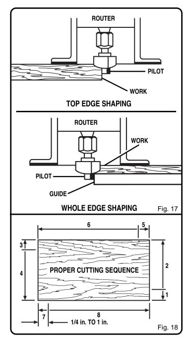
the workpiece edge (the small pilot exposes all of the bit; the large one reduces this amount by 1/16 inch (1.6 mm).
